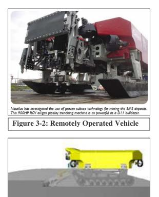
Figure 3-3: ROV with drum cutter
