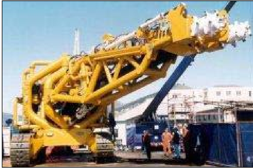
Figure 19-10: 250 tonne Diamond Mining Machine with slewing arm
