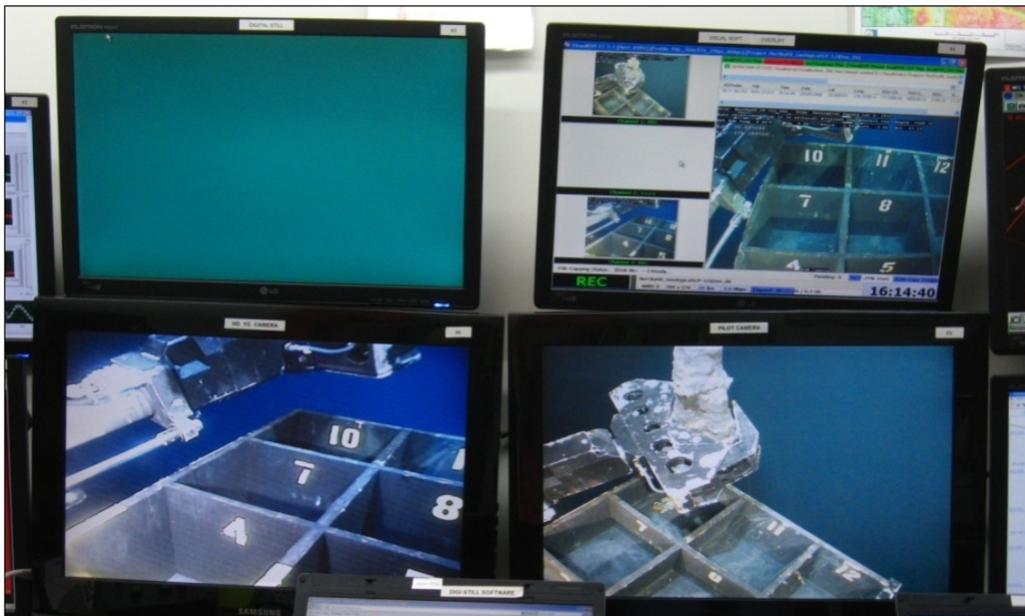
Figure 12-5: Chimney sample 20060 (Tahi Moana 1) being loaded into the 'Geobox'
